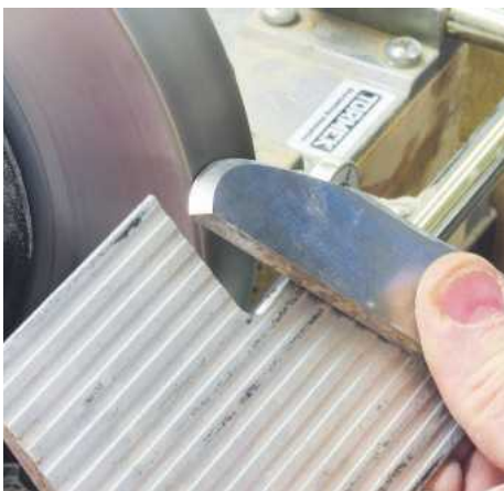
▲ Pic.3 The tool can be used in shear cutting mode by turning the tool on an angle. It's good to soften the lower edge of the tool so it glides effortlessly along the toolrest
